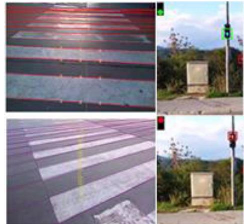
**Fig.5. Crossings and traffic light detector**
