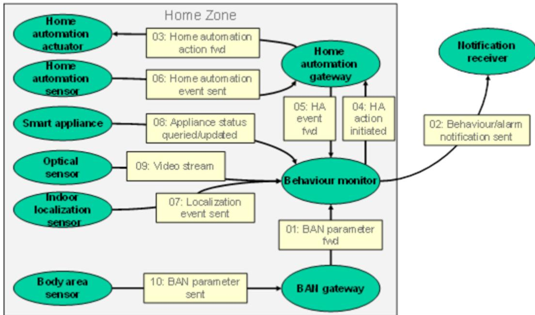
**Figure 4: Actors and Transactions of the Behaviour Monitoring Integration Profile**
