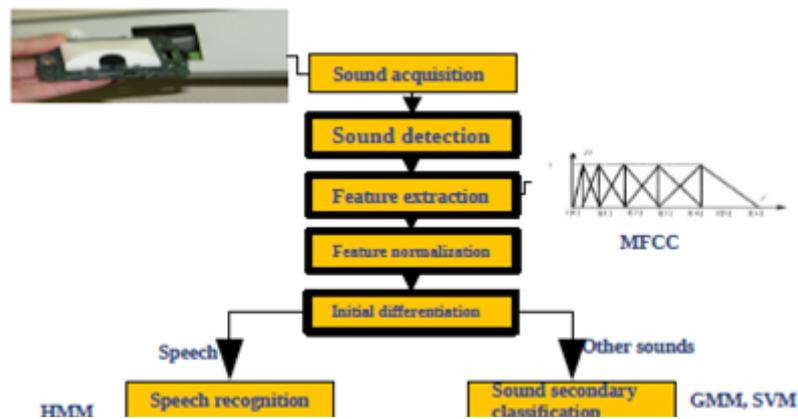
Figure 1: Sound environment analysis architecture
