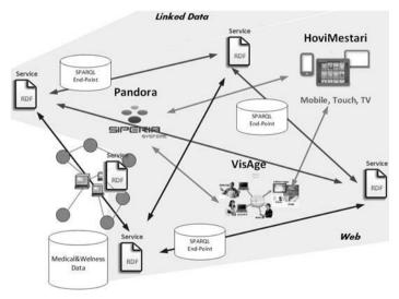
Fig. 2. Decentralised Service Delivery Architecture
