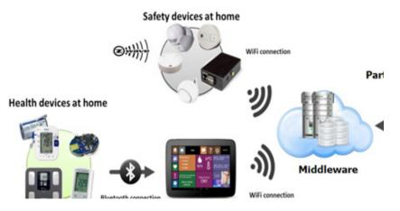
Figure 6 SAAPHO global system architecture
