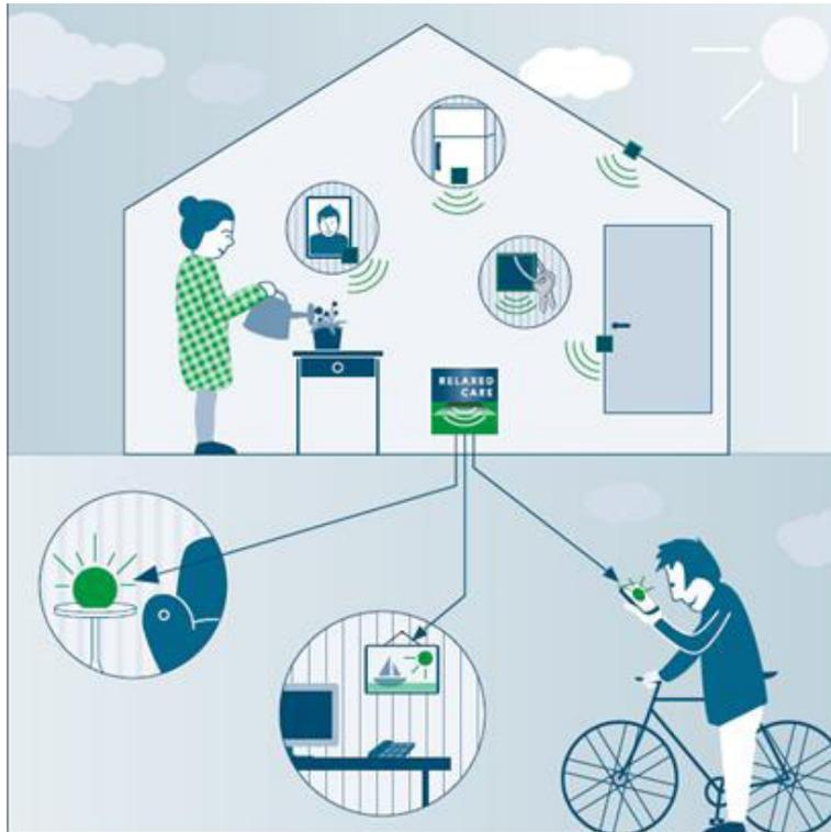
**Figure 13: The image shows the basic concept of RelaxedCare. The upper part of the figure shows the AP at home with various sensors placed throughout the apartment (indicated by the green curved line symbols). The lower part shows the IC with various UI devices, either at home (left, color changing lamp), at work (middle, picture frame) or outdoors (right, smartphone app).**
