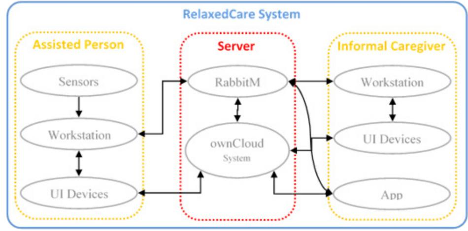
Figure 12: This figure gives an overview of the RelaxedCare System, which can be split up into three distinct subsystems: The AP-side, Server and IC-side
