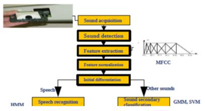
Figure 1: Sound environment analysis architecture
