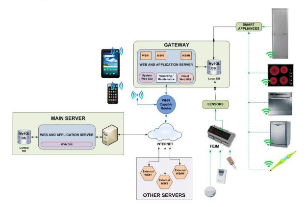
Figure 42 – Food project architecture according to deliverable 3.1
