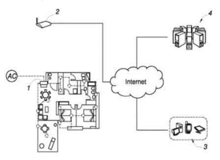
Figure 13 - Scheme of these monitored home appliances and its related cloud computing
