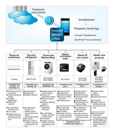
Figure 14 - Panasonic smart appliances scheme; all of them controlled by an Android smartphone and Cloud services
