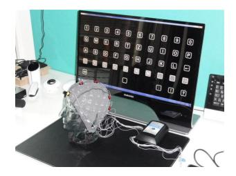
Figure 4: In case the user is unable to use speech or touch inputs, the robot can also be controlled by means of a brain-computer-interface.
