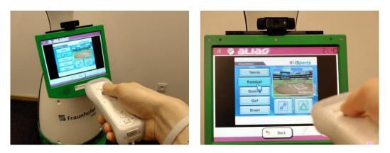
Figure 6: The integrated Wii gaming console module is operated by its proprietary Wii Remote controller. Actual physical movements are reflected in cursor movements on the screen (left.) The Wii Remote control requires a clear line of sight to the sensor array on top of the screen (right.)
