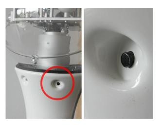
Figure 3: The robot's revised microphone, located at its neck.
