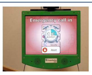
Figure 2: The ALIAS system uses the display unit to notify the user about an eminent emergency call.
