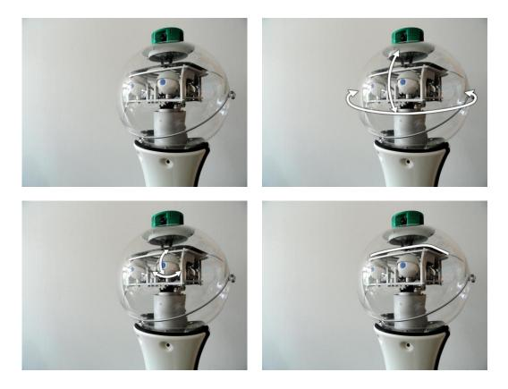
Figure 7: The robotic head (upper left) can be rotated and tilted (upper right). Its eyes can turn sideways and its eyelids can be closed (lower left). On top its eyes an array of LEDs (lower right) may be switched on or made blink in various styles.
