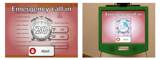
Figure 31: The emergency call procedure is preceded by a 20 second countdown to provide the user with the ability to cancel the process on false alarms.
