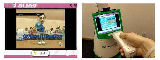
Figure 30: The Wii gaming console, integrated with the GUI (left). Games are played with the special Wii Remote controller (right).
