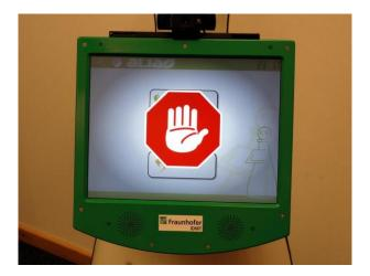
Figure 8: In case the robot is moving, the touch screen unit acts as an emergency stop button.
