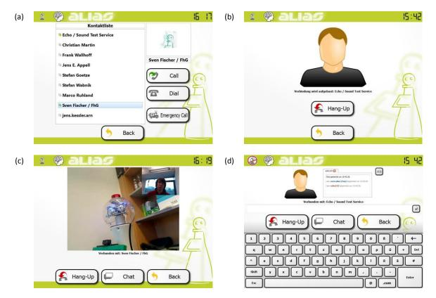
Figure 23: The telephone module in various states: (a) the main screen showing a list of contacts, (b) a call is beeing established, (c) an active video call, and (d) an active chat session (without video.)
