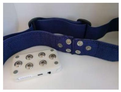
Figure 3 - Snap connectors that allow the textile band to attach to the acquisition unit
