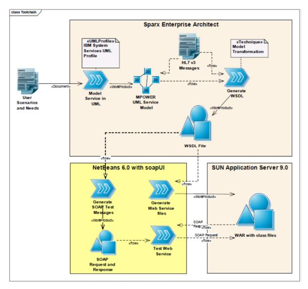
Figure 6: mPower service development tool chain
