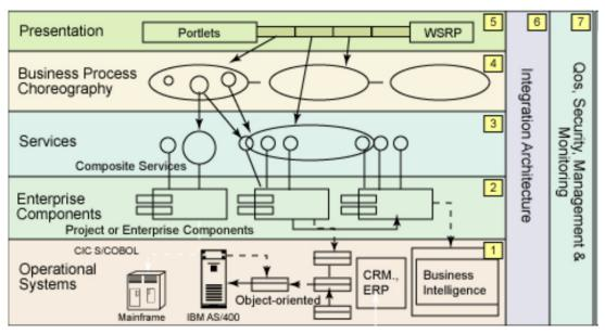
Figure 18: IBM SOA reference architecture
