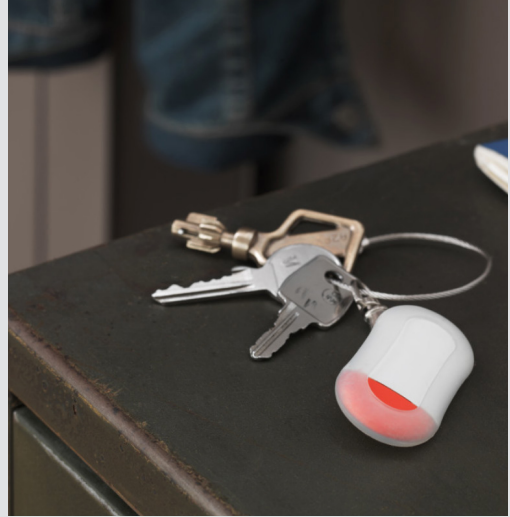
A sensor Cookie attached to the keyholder to monitor who comes back home
