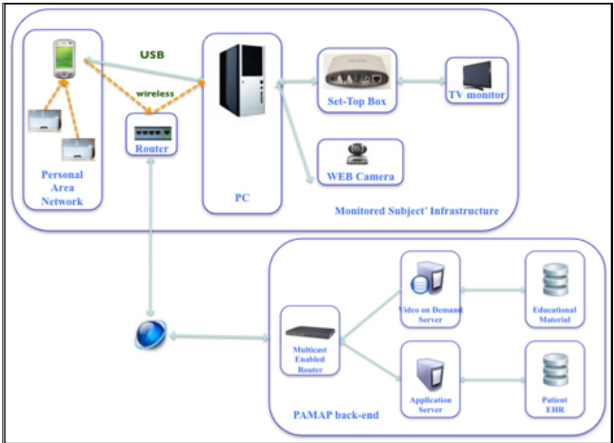
Figure 2: PAMAP Measurement Component Interaction Diagram
