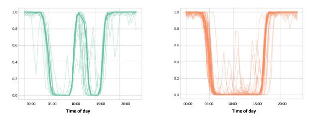
Fig. 6: extraction of different clusters of patterns regarding daily bed usage. Two prototypes are identified: one having the user rest on bed after lunch (left), and one in which the bed is just used in night hours (right).
