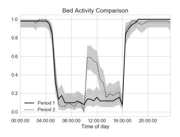
Fig. 5: comparison of bed sensor profiles for two consecutive periods (20 days each). Non-overlapping confidence intervals indicate automatically-detectable, meaningful behavioral changes.
