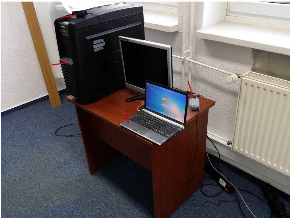
Fig. 2. PIA Integration Site – Room 1 – video server, caregiver laptop, Raspberry Pie unit, Logitech HD camera.
