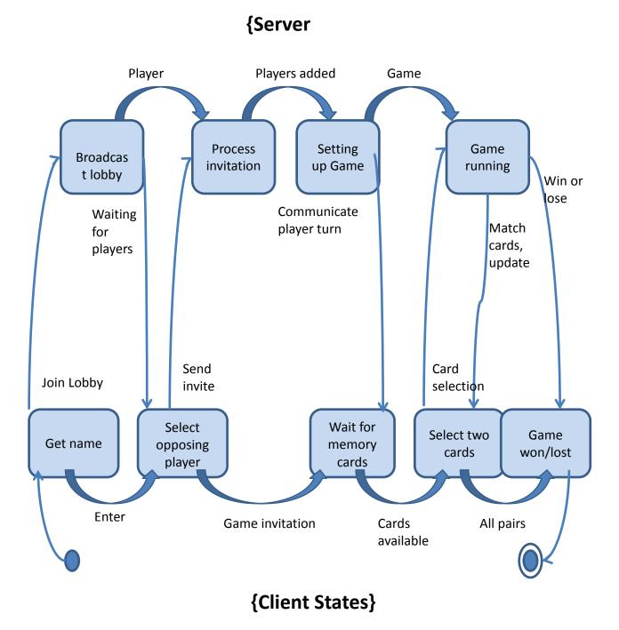
Figure 7. Client/Server state transition diagram
