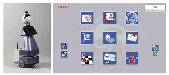
Figure 1: RobuMATE prototype and HCI/HMI main menu on Touchscreen PC (Tablet PC)
