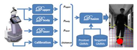
Figure 17 Synopsis of the developed human detection system.
