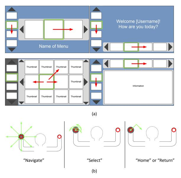
Figure 4: (a) Examples of typical simple menu designs und user interfaces for gesture controlled menu navigation (selected for use in the project) (b) Corresponding selected Deictic gestures for menu navigation.
