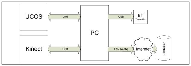
Figure 6 -Block diagram of gesture recognition components
