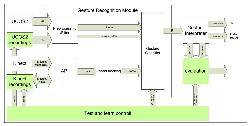
Figure 8: Block diagram of SW components and theirrelationship
