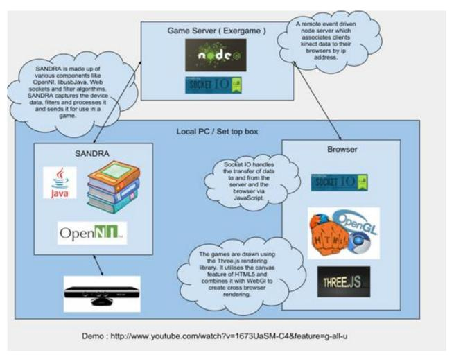
Figure 7: AntiqueHunt System Architecture
