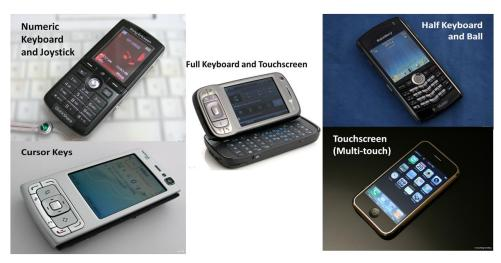
Figure 36. Different input devices
