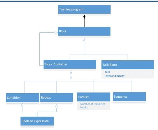
Figure 12: Simplified class diagram of the training program
