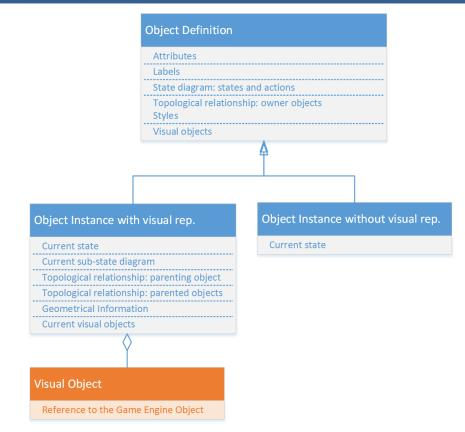
Figure 7: Simplified class diagram of the Object Definition Class, the Object Instance and the Visual Object.
