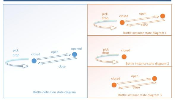
Figure 8: Complete state diagram of the object definition and three possible state diagrams of object instances
