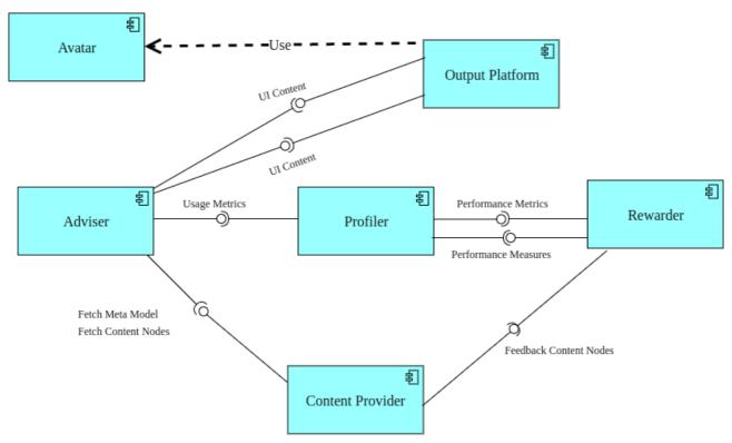
Figure 4: Development View of the Components
