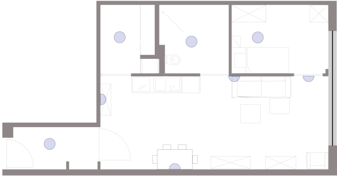
Figure 4: Setup of PIR sensors in flat in Dendermonde.
