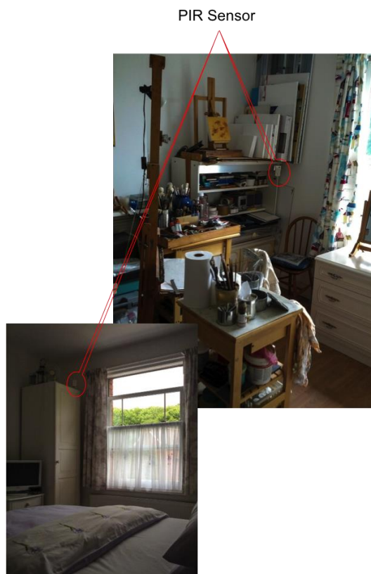
Figure 11: Sensors are glued to furniture
