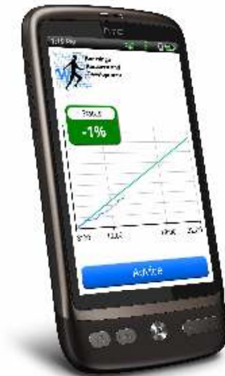
Figure 2: The Smartphone (HTC Desire) showing the graph screen, with reference line (green) and current activity (blue). The status icon shows the activity trend from the past 5 minutes.
