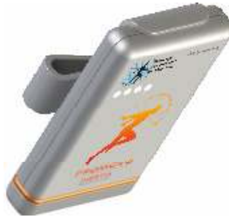
Figure 1: The ProMove 3D wireless inertial sensor, pictured here as a 3D render with an attached belt clip for mounting on the patient's hip.
