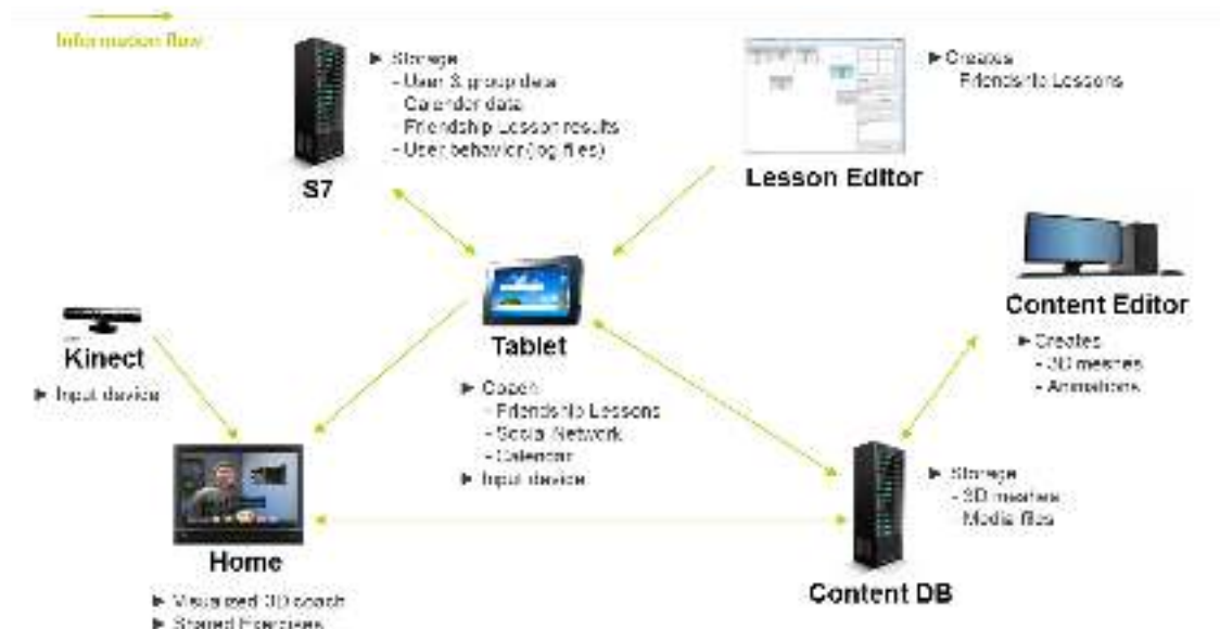
Figure 1: V2me system architecture
