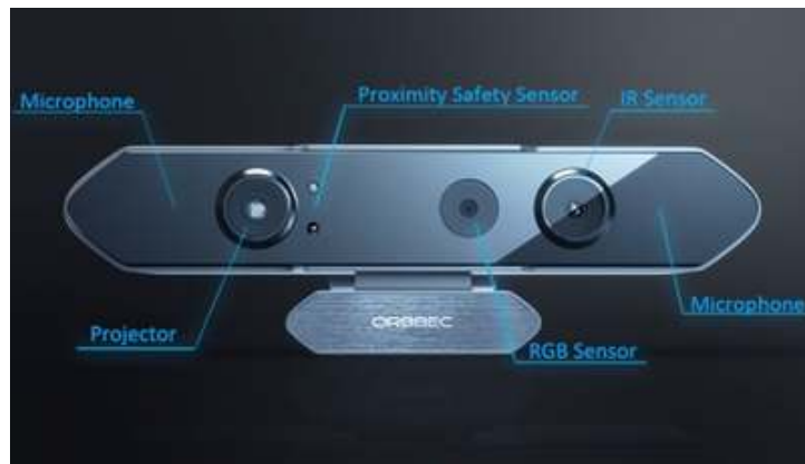
Figure 1.13: The Orbbec Persee depth camera used for the vINCI pilot.
