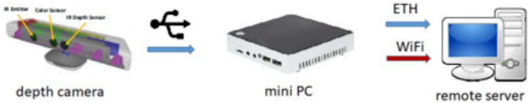
Fig. 2. Connection between the depth sensor and the backend server.
