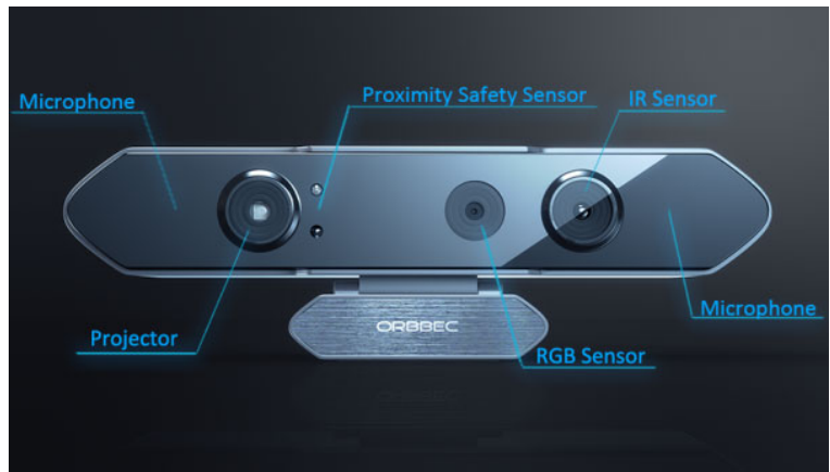
Fig. 11. The Orbbec Persee camera used in vINCI.
