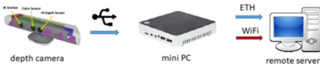
Figure 3.2: Connection of the depth sensor to the remote server.
