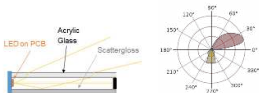
Figure 18: Black Box Concept for the GREAT Uplight (left) and the LID in red (right)
