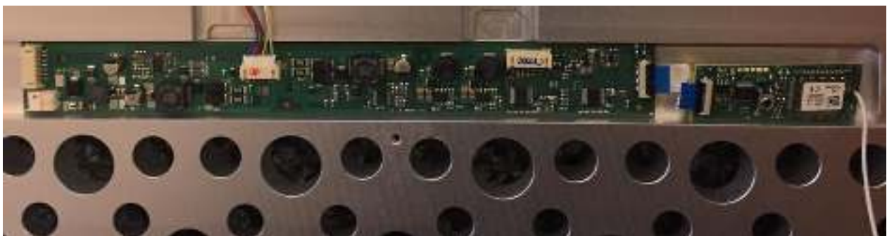
Figure 27: Build-in driving board for controlling Up- and Downlight
