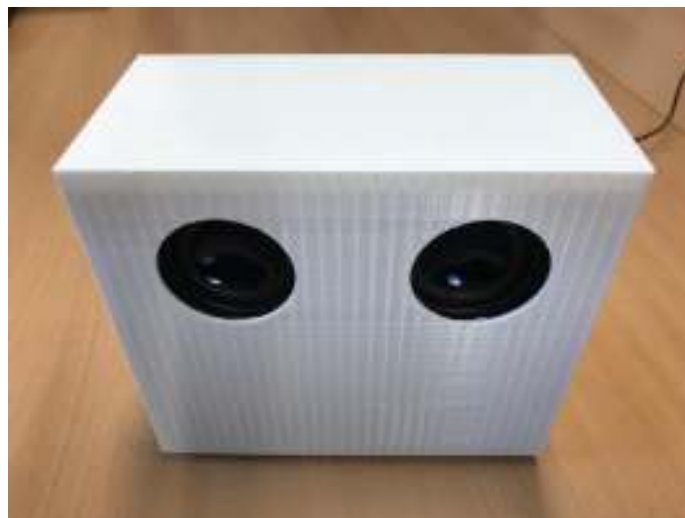
Figure 43: Prototype of sound module in combined housing for the Logitech Z150 speakers.
