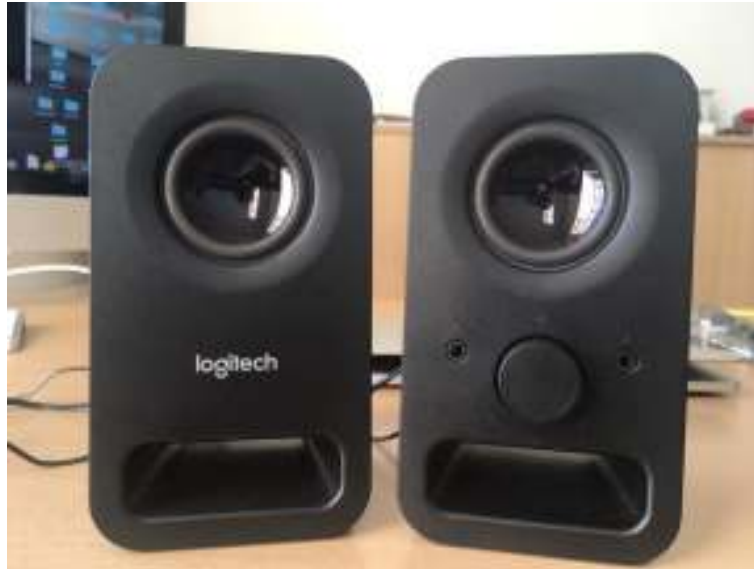
Figure 38: GREAT sound module based on Logitech Z150 active speaker
