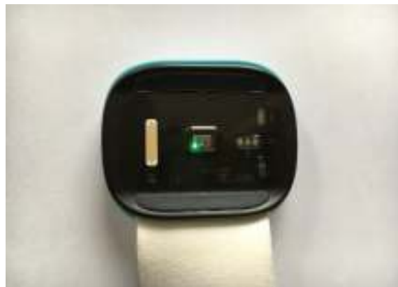
Figure 62: Enverion back with light and galvanic skin sensors
