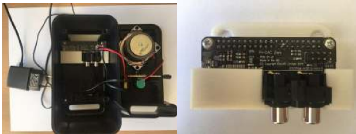
Figure 39: Raspberry Pi and Pi-DAC Zero integrated into the Z150 active speaker.
