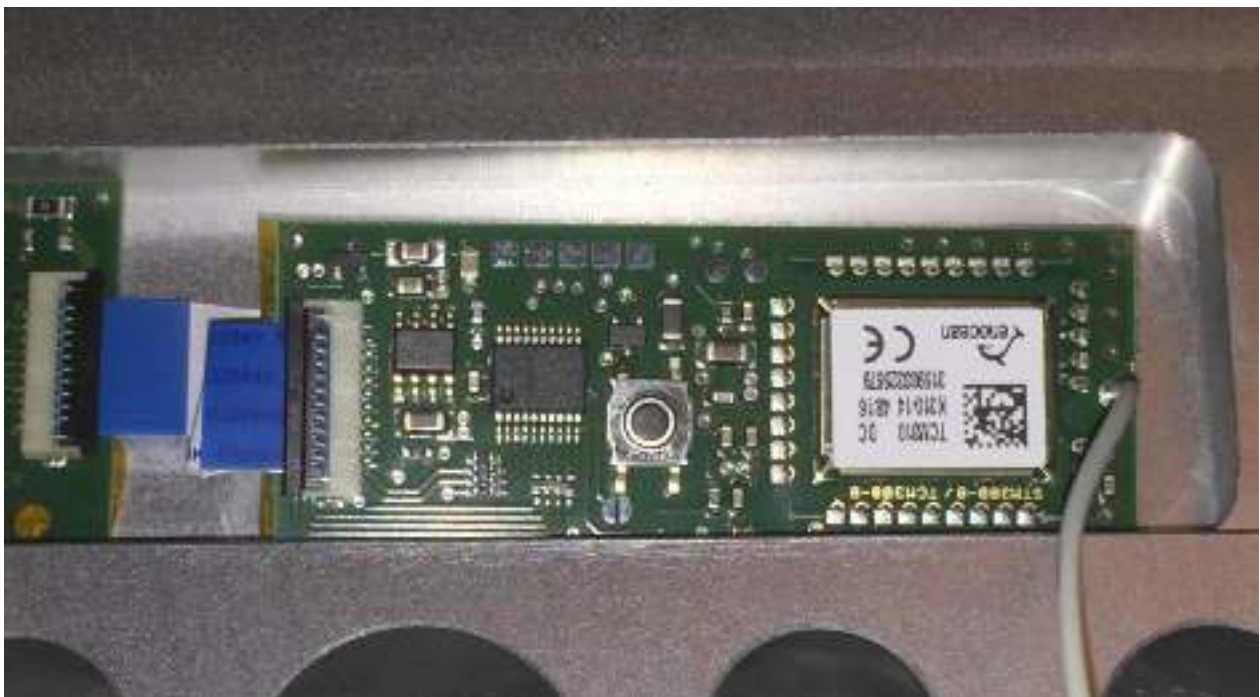
Figure 29: EnOcean communication circuit board for controlling Up- and Downlight
