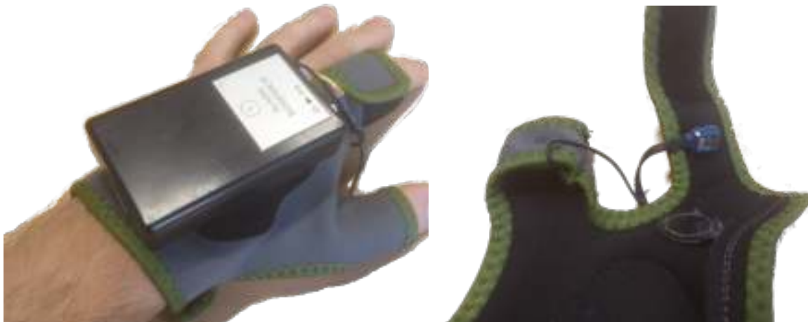
Figure 8: Skin conductance measurement tool: (left) how to wear it (right) it measures the skin conductance between index finger and thumb
