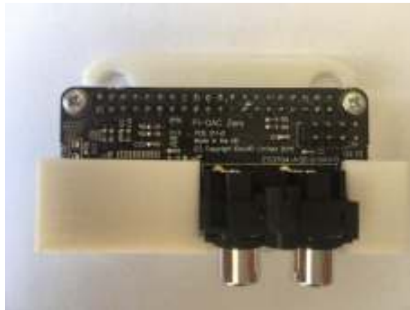
Figure 36: Raspberry Pi and Pi-DAC Zero integrated into the Z150 active speaker.
