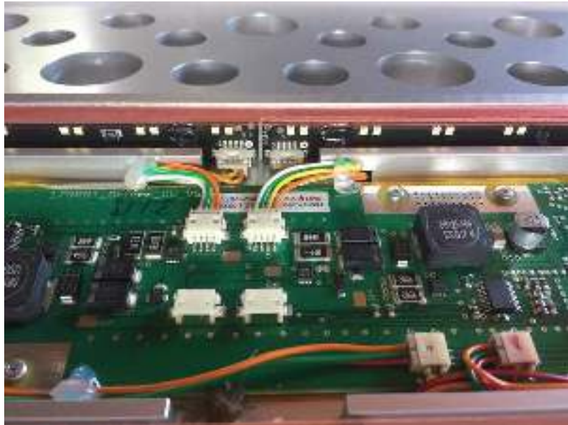
Figure 12: The LEDs are placed on the edge for lateral input of light in the light guiding plate
