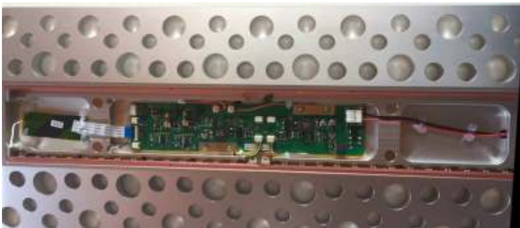
Figure 29: New, optimized luminaire head with EnOcean board and driving board
