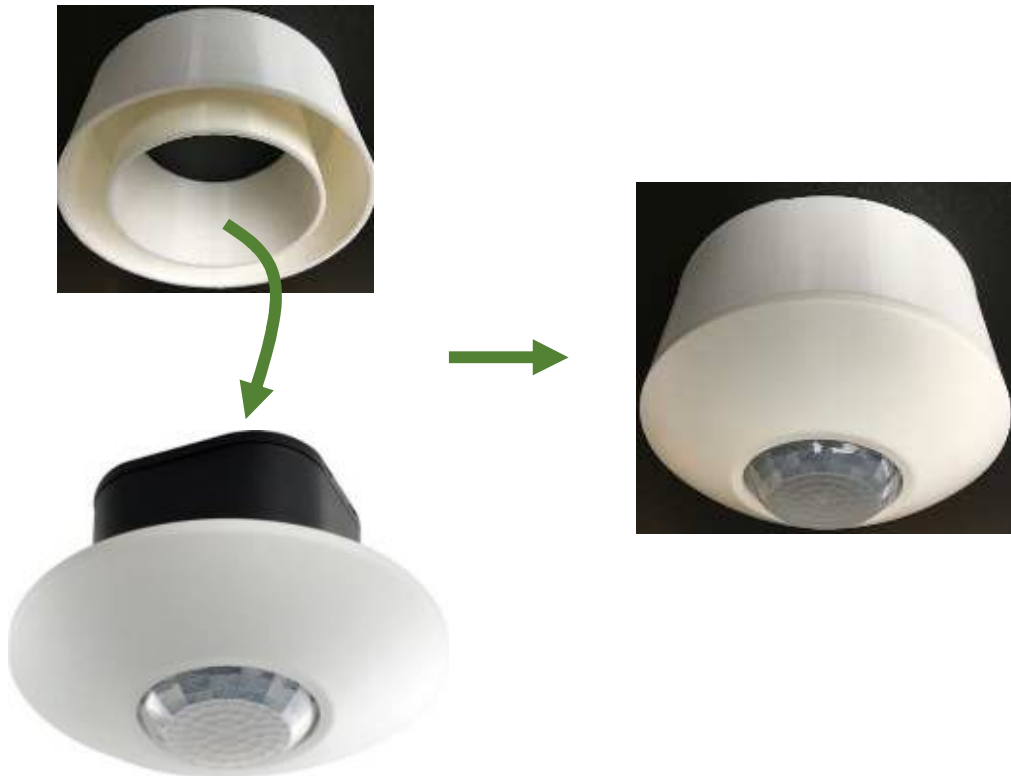
Figure 60: Thermokon SR-MDS BAT with extra light 3D printed cover
