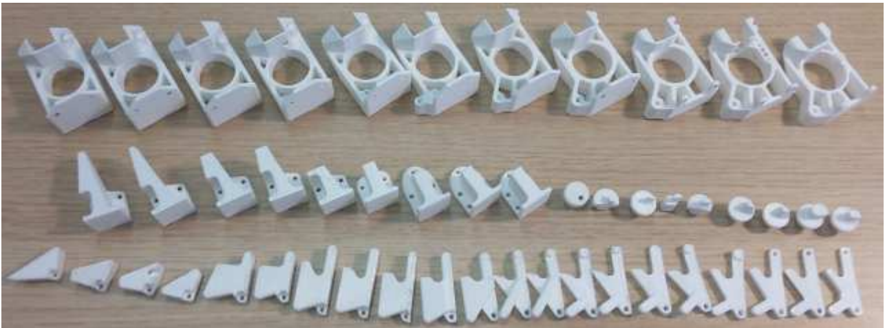
Figure 44: Evolution of mount (top), piston (center left), eccentric (center right) and lever (bottom)
