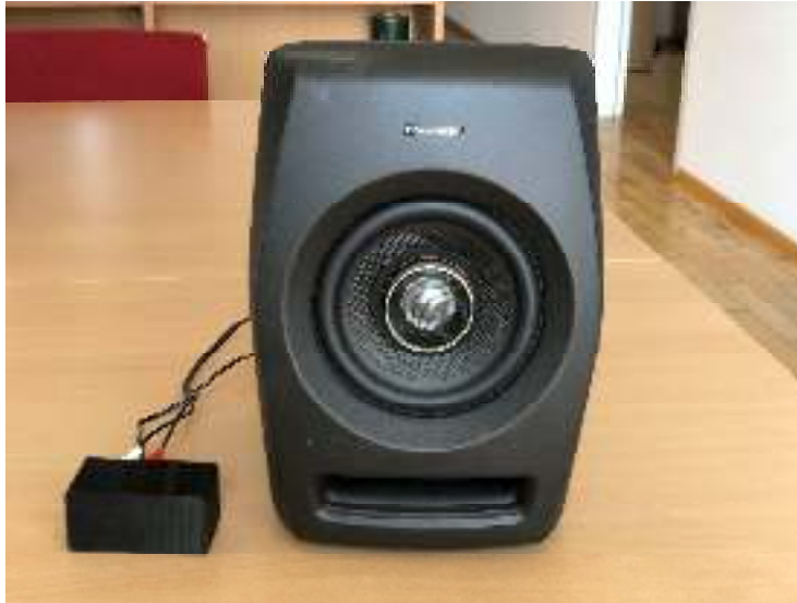
Figure 40: External sound module with a Pioneer RM05 Speaker featuring a frequency range of 40-50.000Hz
