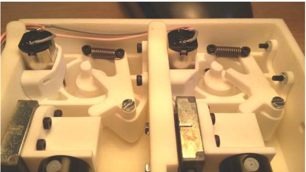
Figure 46: Reworked mechanic installed in the rear casing
