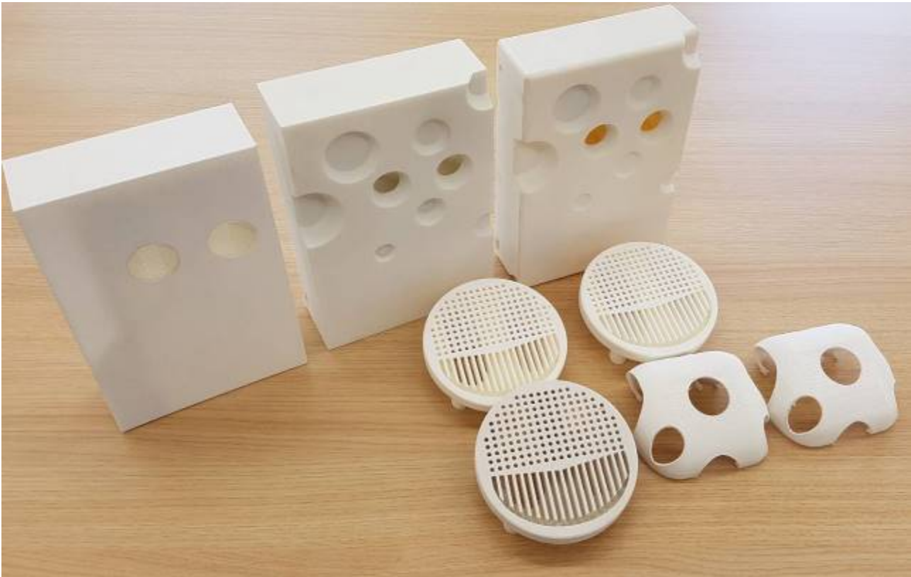
Figure 47: Evolution of the 3D-printed front casing (top) and the two variants of shields (bottom)
