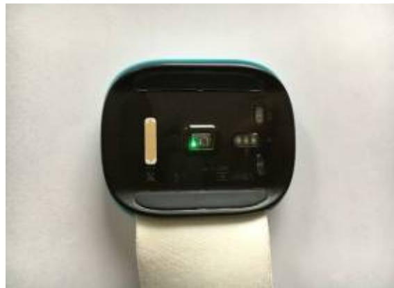
Figure 62: Everion back with light and galvanic skin sensors
