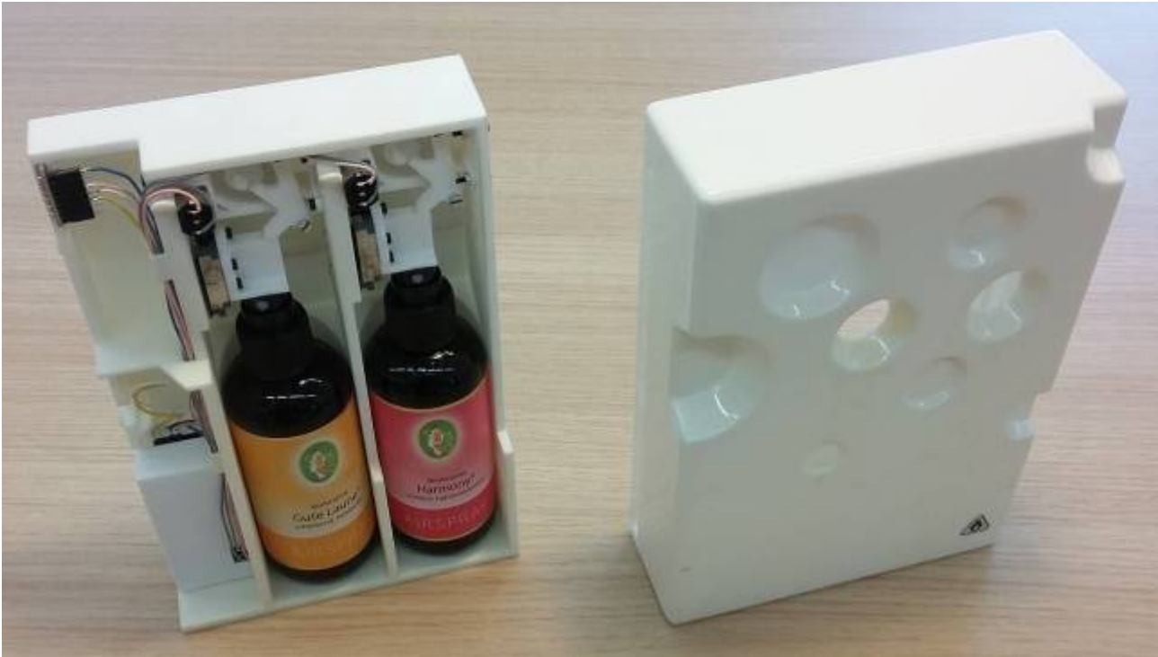
Figure 48: Left shows the completely mounted rear casing, right shows the front casing
