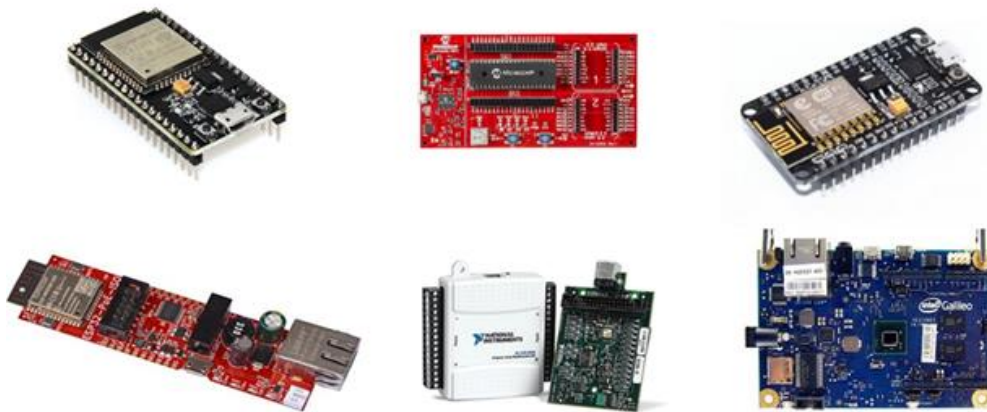
Figure 1 - Examples of OSHD boards (ESP 32, Microchip, NodMCU, OLIMEX PoE, National Instruments USB-6003, Intel Galileo)
