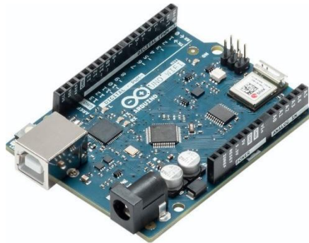
Figure 17 - Arduino UNO Wi-Fi Rev2 (microcontroller Atmega 4809) Source: https://www.arduino.cc/Products
