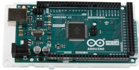
Figure 14 - Arduino Mega (microcontroller Atmega 2560) Source: https://www.arduino.cc/Products
