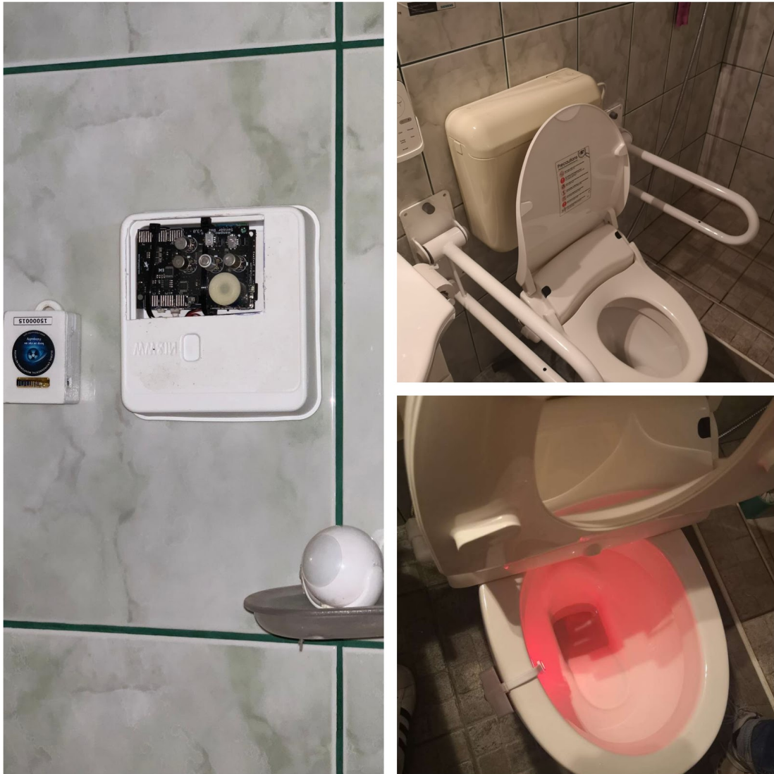
Figure 10: Test site in Romania: Box with electronics for air quality measurement (left), toilet with bidet seat and support bar (upper right) and toilet with UV lamp (bottom right)
