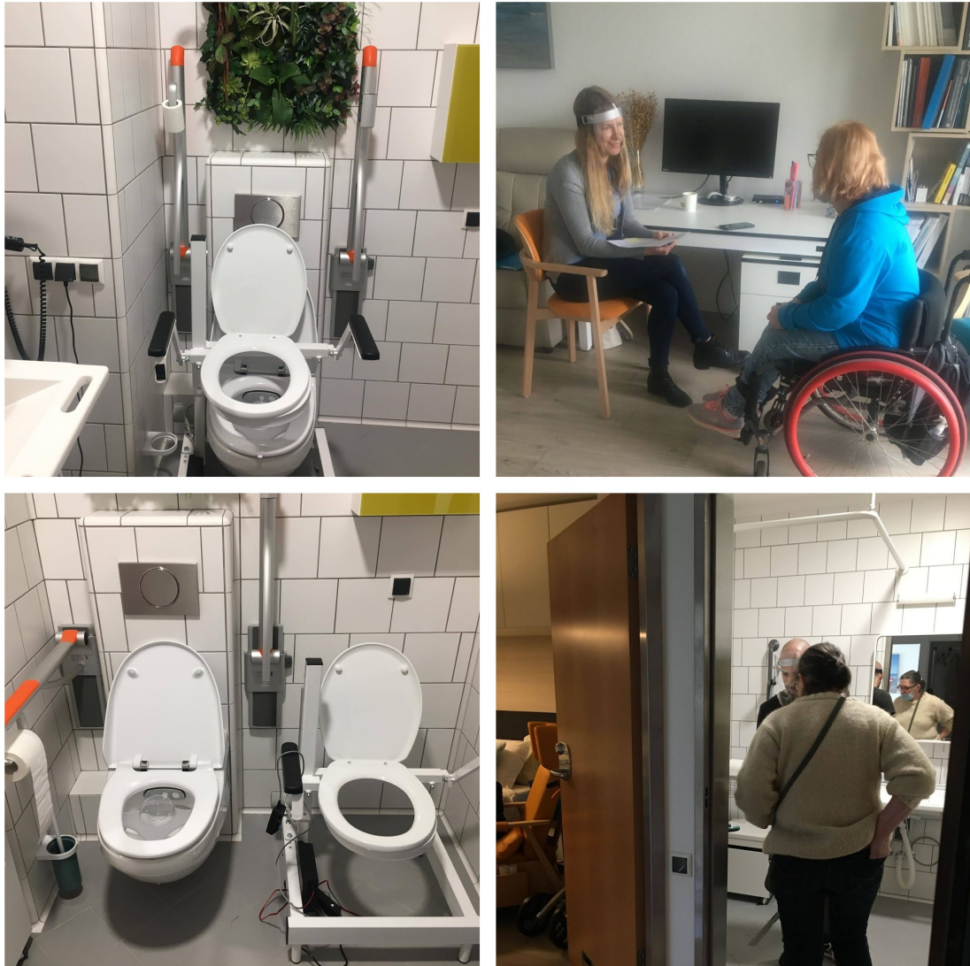
Figure 9: The testing in Poland. GEBERIT AquaClean 8000 with an additional PW GAMA lift next to it (top left) and installed on the existing toilet (bottom left). Participants of the testing - a primary user during the interview with the OSF team member (top right) and caregiver visiting the restroom (bottom right).
