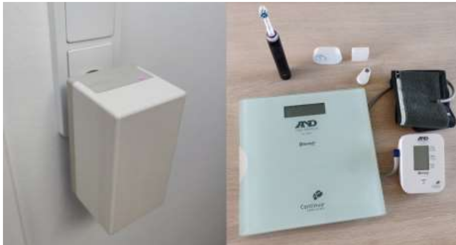
Fig. 11. The CARIOT gateway is marketed by Danish companies Aliviate and Medica Connect, but both hardware and software stack can be licensed to third-parties. It is essentially a platform rather than just a gateway, and can both communicate with local medico and ambient sensor devices, store the data, provide end-user warnings and signaling (via light and sound interfaces), as well as perform long-range communicate using Lora, GSM (2G), 3G/4G/5G, and WiFi. The software stack is flexible, and besides Lora and IP communication, HTTP/HTTPS/REST/MQTT is supported out of the box to any end-point. Some models have support for ZigBee, while BLE and Bluetooth is fully supported. As shown on the illustration, we have used the gateway with toothbrushes, blood pressure and weight devices, as well as presence and occupancy sensors.
