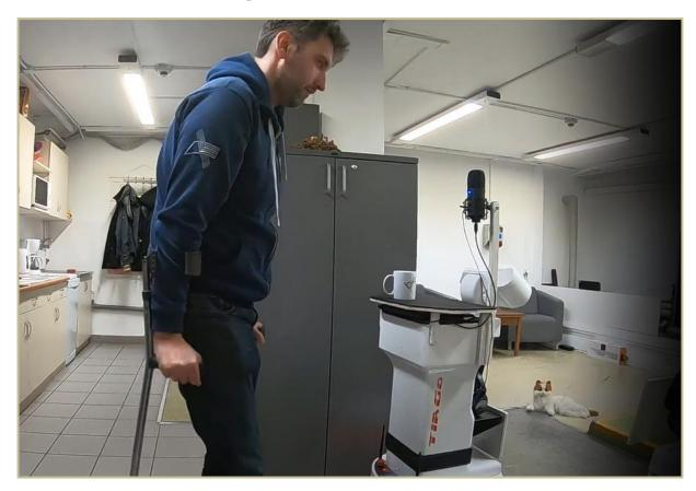
Figure 17 - Tiago helping a person using crutches to transport a cup of tea.
