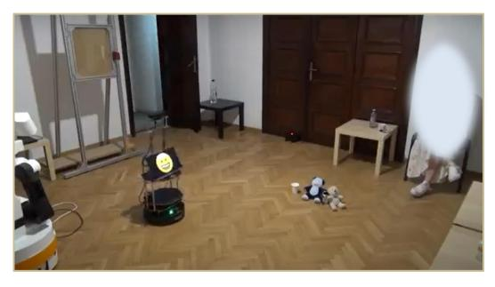
Figure 19 - Turtlebot recognizing objects on the floor and interacting with a user.
