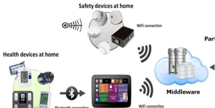
**Figure 6 SAAPHO global system architecture**
