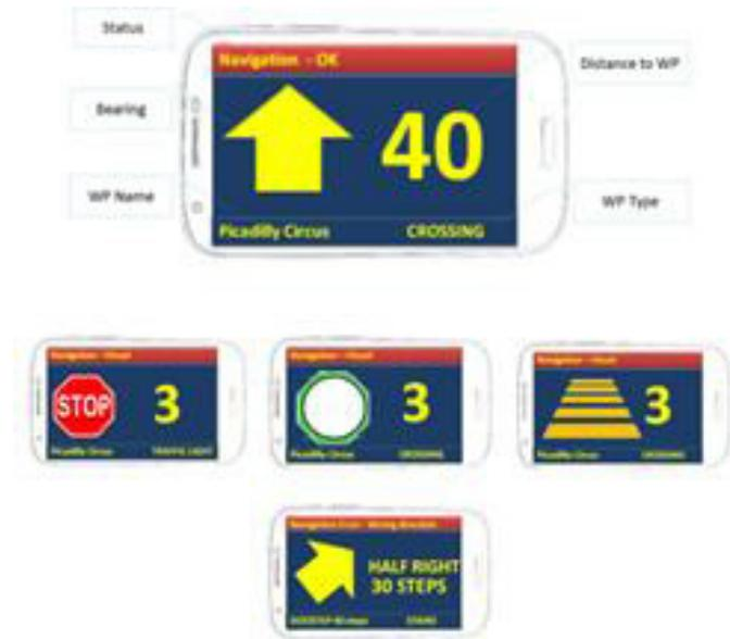
**Fig.6. Human machine interface**
